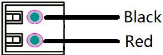
CH3.96mmInterface plug-in anode 2 bits
